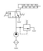
Two Position, Three Way Manually Actuated Spring Offset, DCV
