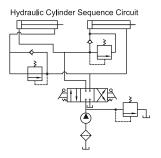
Left Cylinder extends completely and then Right Cylinder extends.
