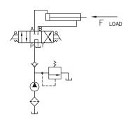
Three Position, Four Way Manually Actuated Spring Centered, DCV
