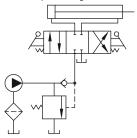
Unloading valve, unloads the pump at the ends of retracting strokes
