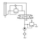
To keep vertically mounted cylinder in upward position while pump is idling.
